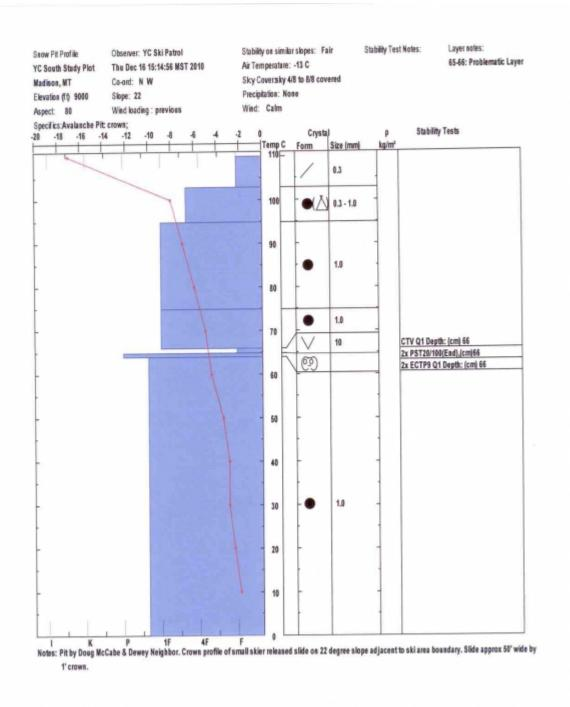
This snowpit is from a skier triggered avalanche near Big Sky on a 22 degree slope. The snowpack is mostly strong dense snow except for a very weak layer of surface hoar sitting on top of a crust about 17 inches down. Pit image: YC Ski Patrol
