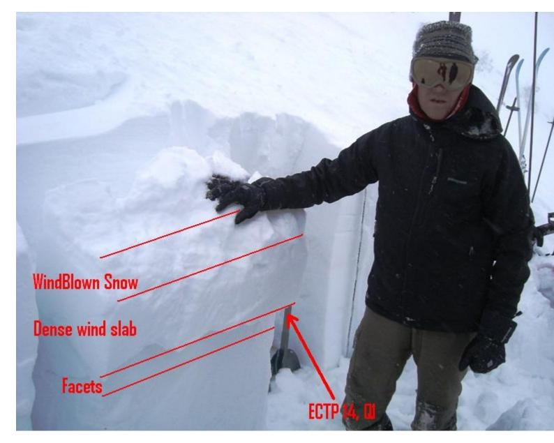
A pencil hardness (very dense) wind slab is sitting over weak, unstable facets. The instability was worse than we were expecting (CT4,Q1; ECTP14,Q1). Skier compaction will NOT effect this weak layer. We will be tracking it closely, but it looks like it'll last a while. Watch the Saddle Peak video (12/17/09) to learn more.
