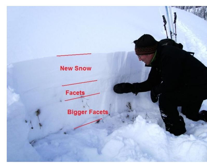
Karl Birkeland checks out the layering in a snowpit at Lionhead in the southern Madison Range. New snow is sitting on large, sugary, faceted grains. This pit was 20 feet uphill from an avalanche that released in the storm. It broke on the new snow and facet interface.
