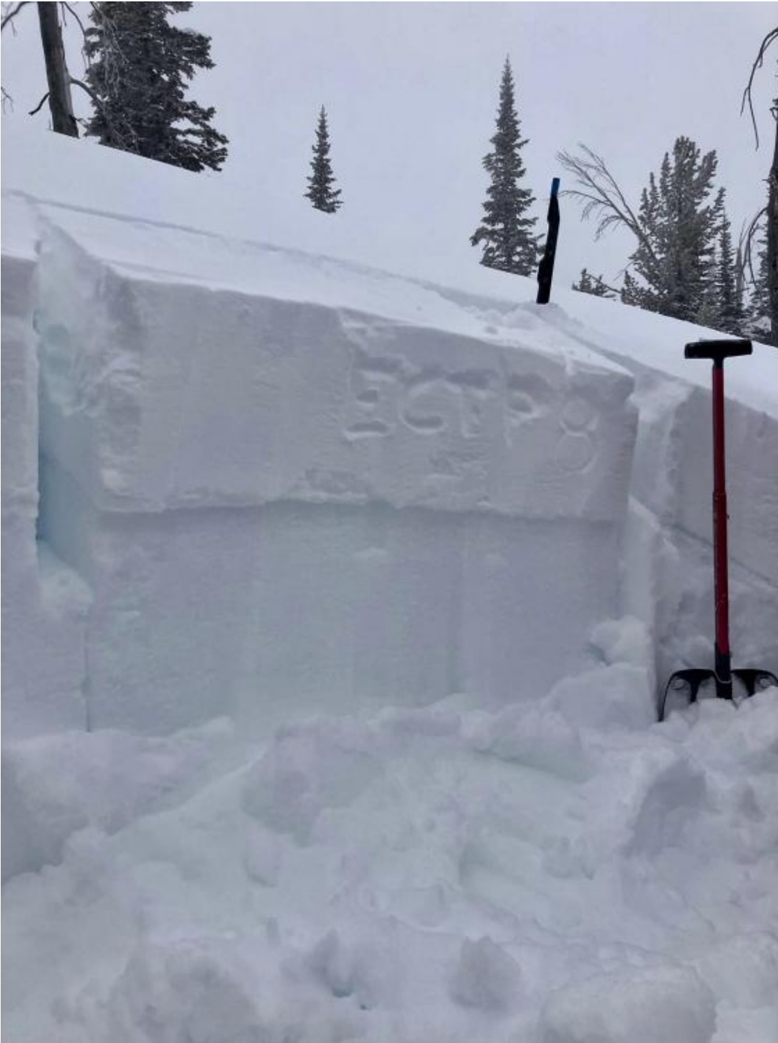
A layer of nsf's and surface hoar was failing ~10 inches deep producing easy ECTP's
